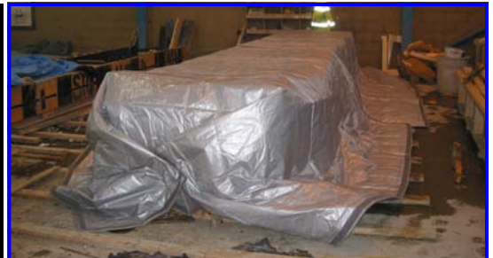
Bi-directional extending duvets shown deployed, both individually and linked together, in a typical ever-changing 'precast' production environment
