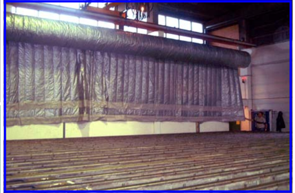
A 'bespoke' 75m x 30m duvet, roll-mounted for single action deployment over the entire production area
