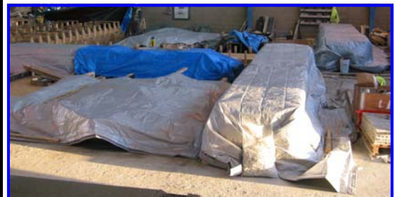
Bi-directional extending duvets shown deployed, both individually and linked together, in a typical ever-changing 'precast' production environment
